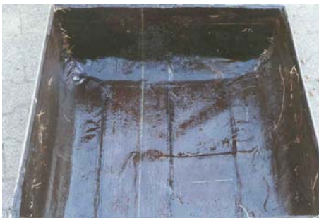
INSIDE VIEW OF THE CONTAINERS AFTER 4 YEARS
